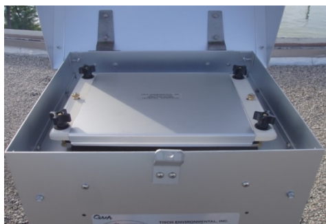
Figure 8.2. Large format (25.4 cm x 20.3 cm) filter holder and filter holder with the cover.
