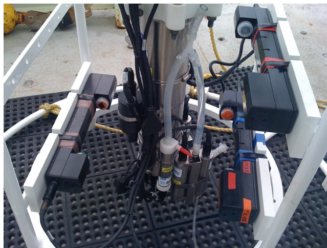
Figure 10.1. Mounting of 2 transmissometers and PIC sensor on the GEOTRACES rosette system during the 2008 and 2009 Intercalibration Expeditions. Plastic caps prevent optics contamination see section 10.1.3 . Methodology from Bishop and Wood (2008).
