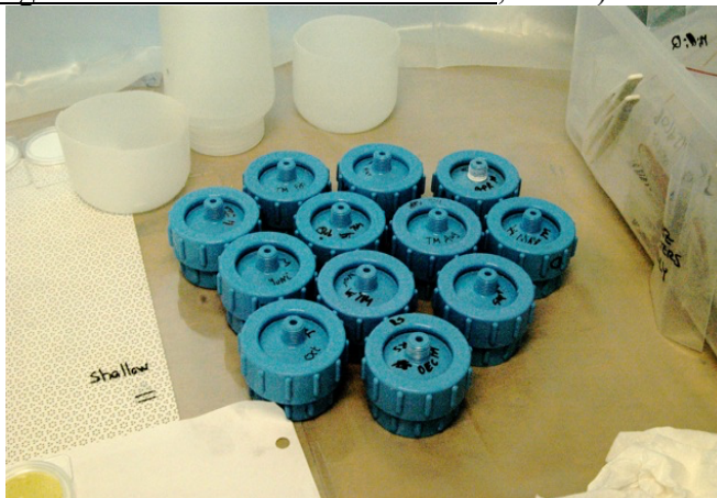
Figure 7.4. Advantec-MFS polypropylene 47 mm filter holders.
