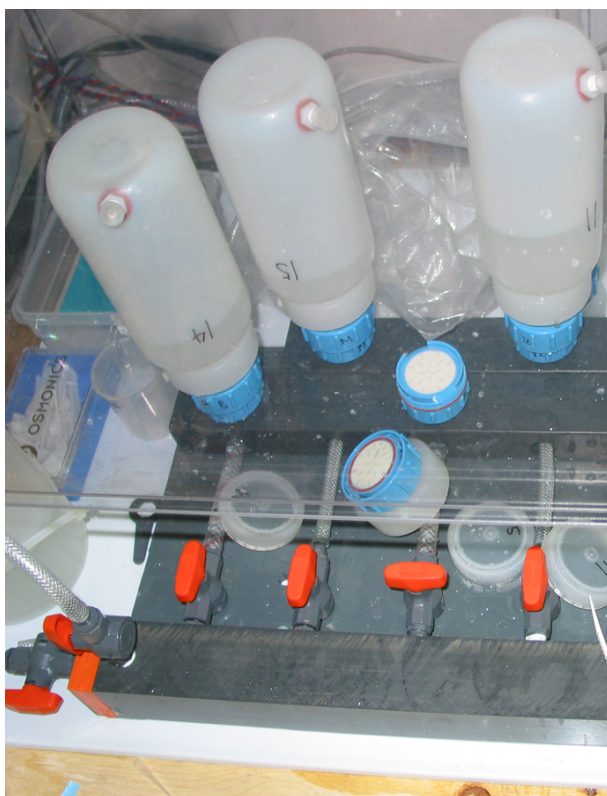
Figure 7.7. An example of a 1 L offline filtration method as used routinely on CLIVAR A16N, A16S, VERTIGO, and GEOTRACES IC expeditions. Pre-cleaned 1L LDPE bottles are modified with closing air vents at bottom. Sample is quickly transferred from the GO-FLO into the 1 L LDPE bottle which is then capped conventionally. Once returned to a Laminar Flow bench environment, the top is substituted for a tapered adaptor which has a mated 47 mm MFS filter holder with preloaded 0.45 \mu\text{m} Supor filter. The upstream orifice of the filter holder has been drilled out to twice standard diameter to minimize air-lock effects. Once samples are filtered under 25 to 40 mm Hg vacuum, they are transferred directly to sample bottles for further processing. Primary sample bottles and filter holders are reused after TM-clean DI water rinsing. More information available from J. Bishop ( jkbishop@berkeley.edu ) or Todd Wood ( tjwood@lbl.gov ).
