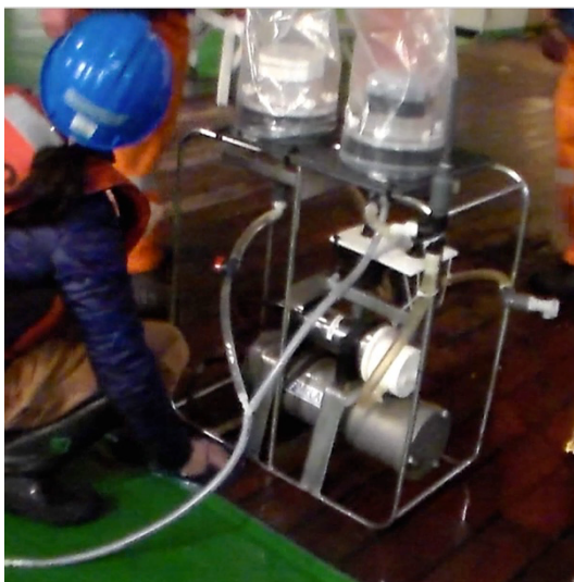
Figure 7.12. On-deck evacuation of seawater from filter holder headspace using vacuum lines to an aspirator pump on deck.
