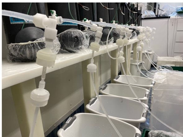
Figure 7.3. Example of collecting size fractionated particles ( 5 and 0.45\ \mu\text{m} ) from GO-FLO bottles.
