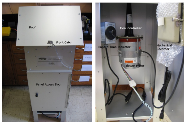
Figure 8.1. Tisch Environmental (TE-5170V-BL) TSP sampler.
