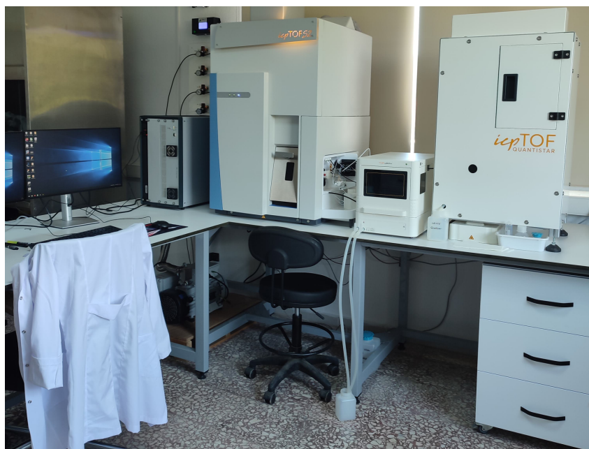
Figure 2: TOF-ICP-MS (icpTOF) with online microdroplet system (Quantistar).
