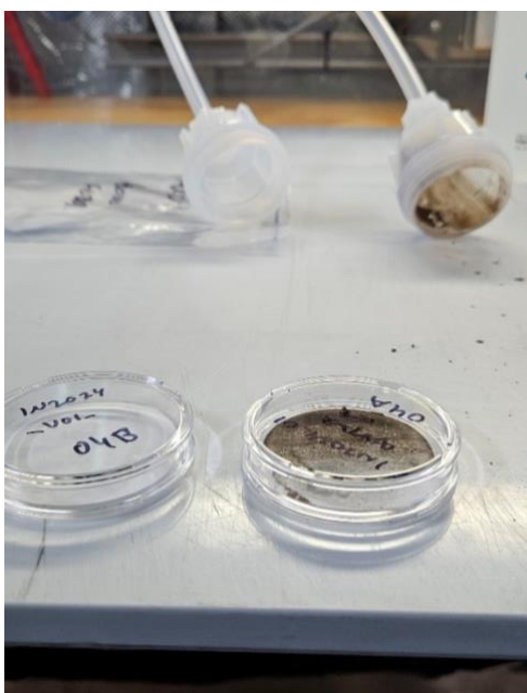
Figure 6: Contamination of aerosol sampling equipment from faulty manifold.
