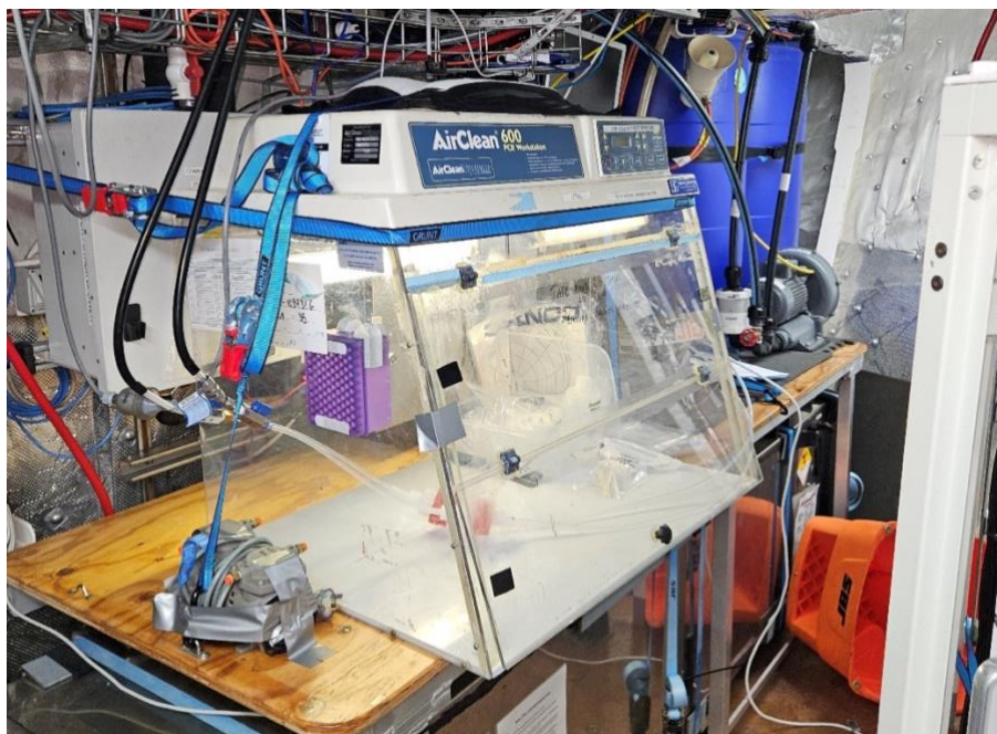
Figure 4: Aerosol sampling manifold in forward aerosol lab.
