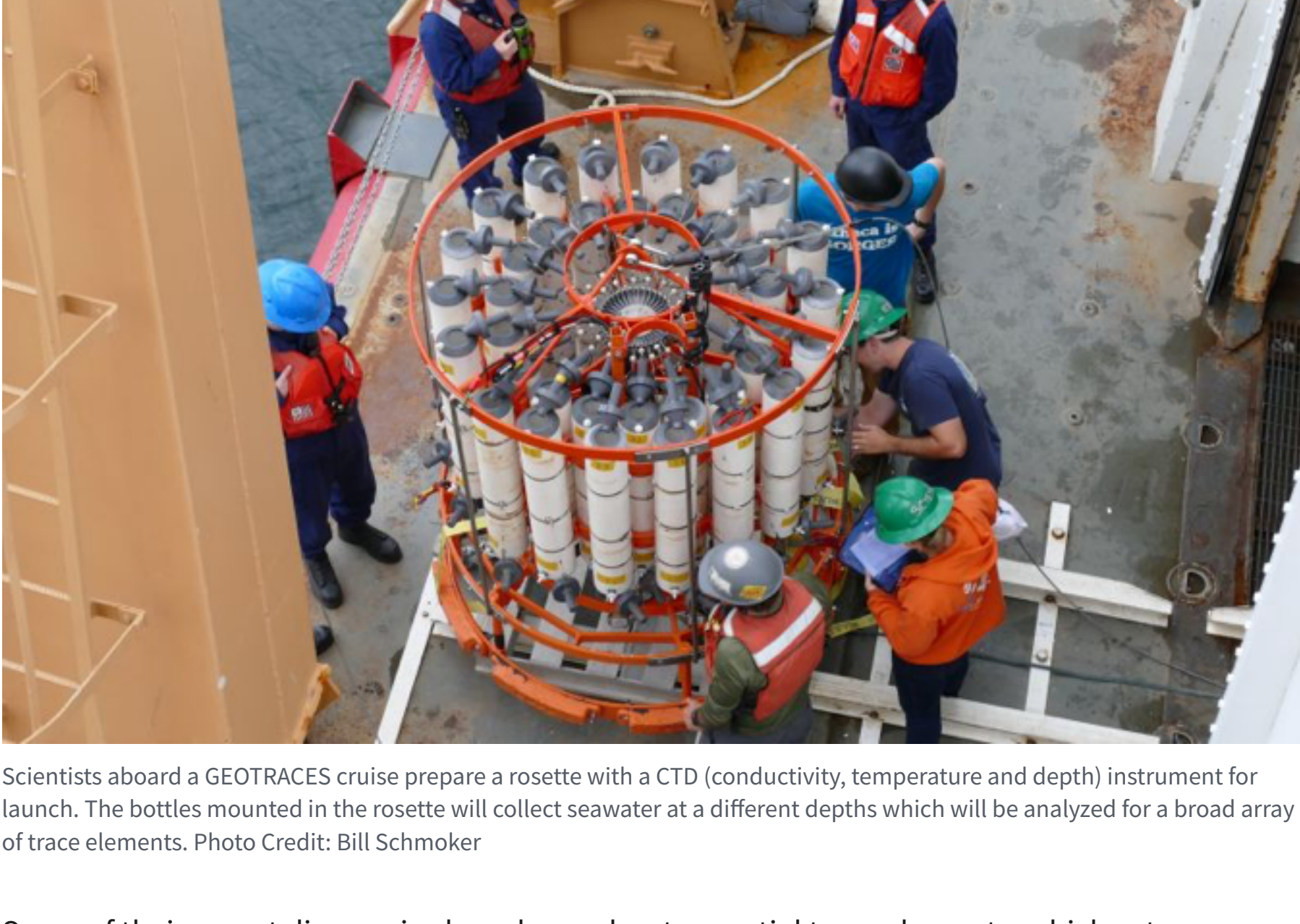
Scientists aboard a GEOTRACES cruise prepare a rosette with a CTD (conductivity, temperature and depth) instrument for launch. The bottles mounted in the rosette will collect seawater at a different depths which will be analyzed for a broad array of trace elements. Photo Credit: Bill Schmoker
