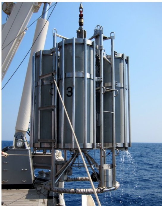
Fig. 6. 2. 2. 1. Photograph of the large-volume water sampler used in the KH-17-3 cruise.
