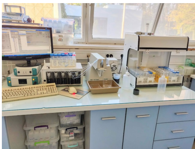
Figure 1. Voltammetric system for automatic determination of trace metals in natural waters
