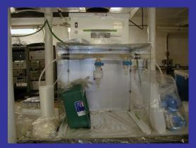
Clean bench with filtered and unfiltered clean water taps from fish/pump supply
