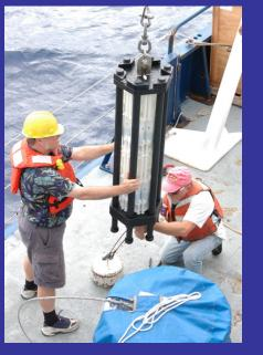
Ed Boyle's MITESS samplers. The vane sampler on the left is used to collect an individual smaller sample. The sampler on the right is used to collect multiple samples to either provide a larger volume or used with a timer to collect at multiple depths. Funding for participation is pending.
