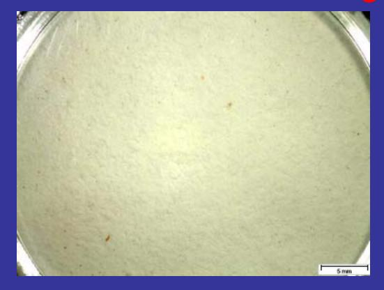
Due to the heterogeneity seen here, we will be distributing replicate whole filters rather than sub-sampling from one filter.
