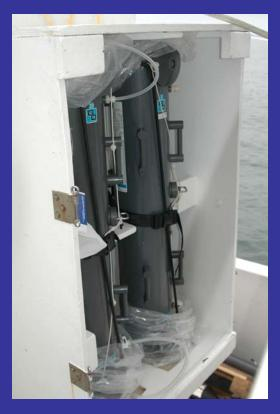
Sampling with 30-Liter GO-Flo samplers - teflon coated, modified, deployed on Kevlar hydroline, tripped with teflon messengers, and with our own winch (Bruland et al. 1979). A "proven" method, but unfeasible for the **GEOTRACES** Program.
