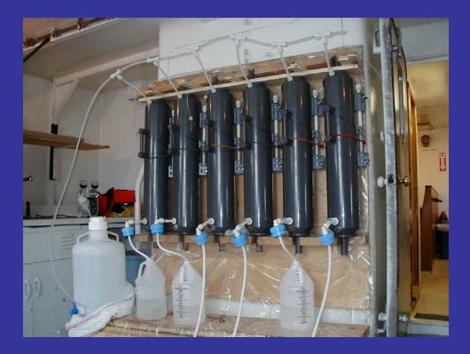
Filtration from Niskin bottles. A similar system will be used with the GEOTRACES GO-Flo bottles (direct pressure filtration), and filter pore sizes and materials will be examined.
