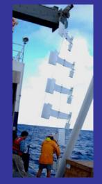
Jingfeng Wu's sampler based upon a modification of the original MITESS ATE/vane sampler that Ed Boyle developed. Funding for participation is pending. • To conduct the intercalibration for GEOTRACES TEIs, we will use two 500 liter tanks and a clean van. We plan on surface and deep composite samples.
