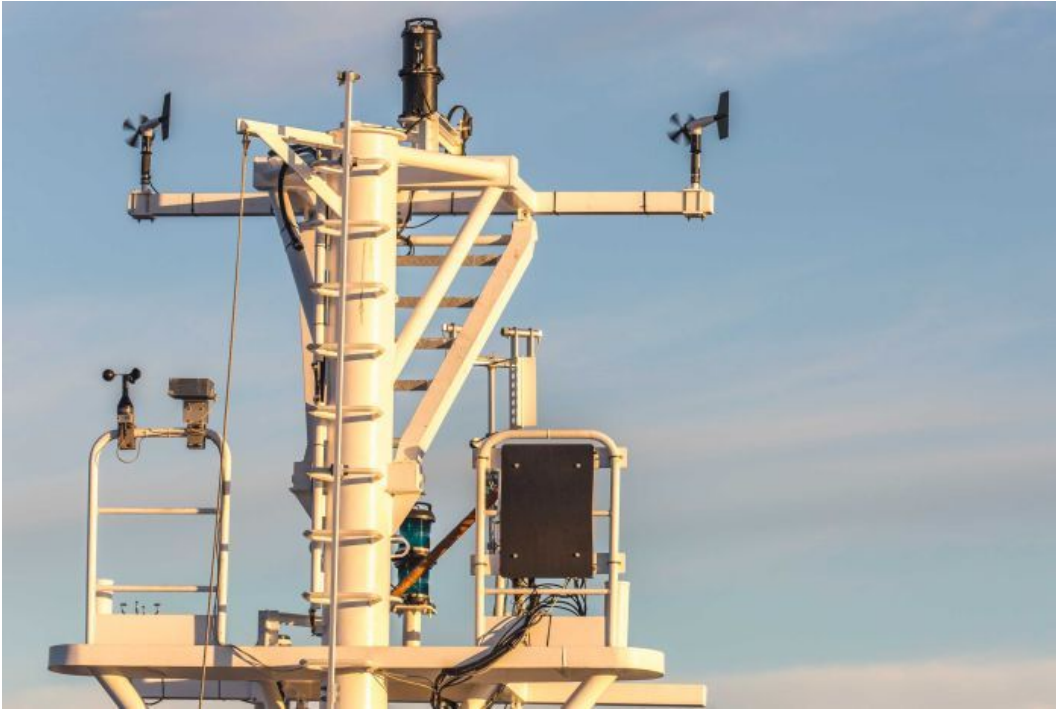
PHOTO: The equipment on the mast includes a clean air intake system. (ABC RN: Ann Jones)
